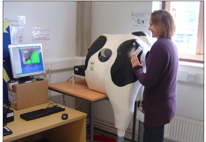
Fig. 26: University of Queensland veterinary student Dr Bryony Dixon practices pregnancy diagnosis using a haptic bovine rectal palpation simulator at England's Royal Veterinary College in 2008
